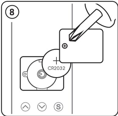
**8. Insert or replace the button cell battery**
